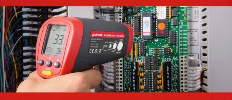
The Beha-Amprobe series of infrared and contact thermometers are a complete line of high performance diagnostic tools designed for HVAC/R, electrical, industrial maintenance applications.
